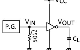
$I_{CC(\text{opr})}$  TEST CIRCUIT
