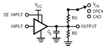
$C_L$  includes load and stray capacitance
