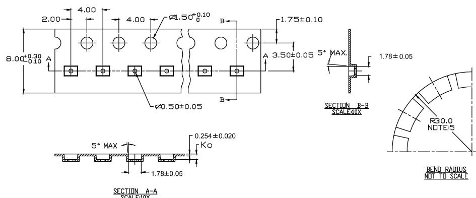
**Tape and Reel Specification** (Continued)**REEL DIMENSIONS** inches (millimeters)
