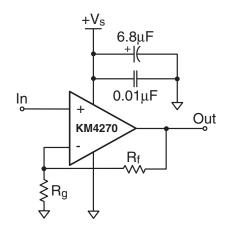
**Notes:** 1) For +5V supply, a  $2V_{pp}$  condition was used. 2) For G = +1, R<sub>f</sub> = 0.
