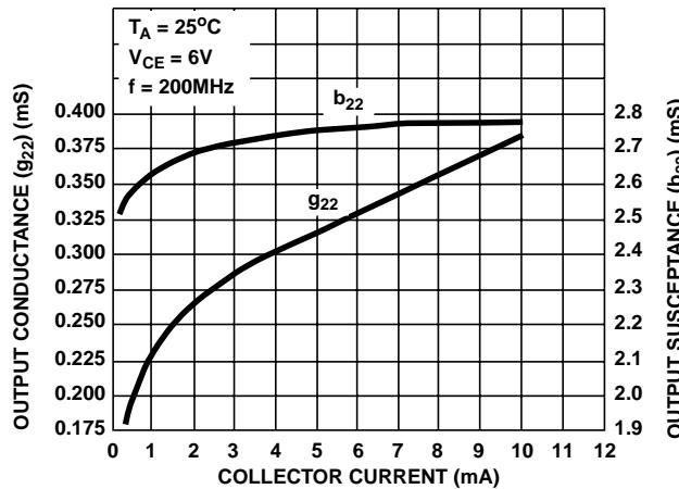
FIGURE 15. OUTPUT ADMITTANCE ( $Y_{22}$ ) VS COLLECTOR CURRENT
