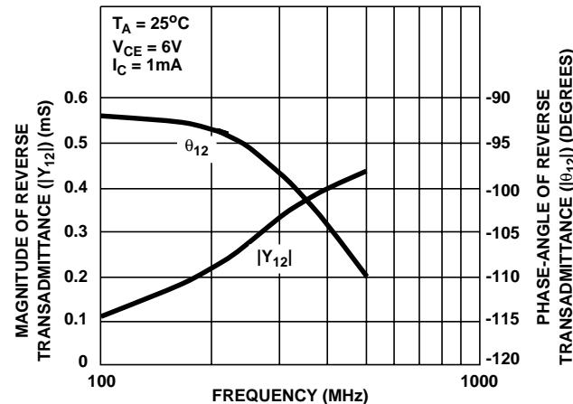
FIGURE 19. REVERSE TRANSADMITTANCE ( $Y_{12}$ ) VS FREQUENCY
