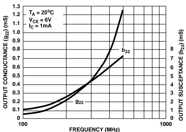
FIGURE 14. OUTPUT ADMITTANCE ( $Y_{22}$ ) vs FREQUENCY
