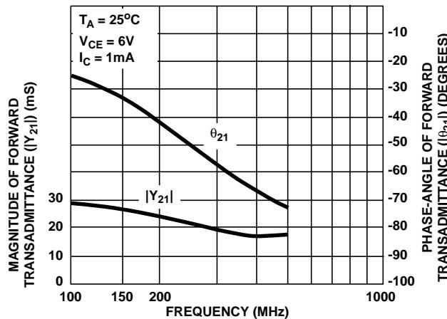
FIGURE 17. FORWARD TRANSADMITTANCE ( $Y_{21}$ ) VS FREQUENCY
