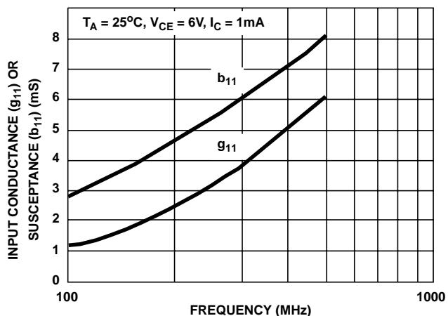
FIGURE 12. INPUT ADMITTANCE ( $Y_{11}$ ) vs FREQUENCY
