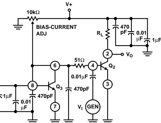
FIGURE 1. VOLTAGE-GAIN TEST CIRCUIT USING CURRENT-MIRROR BIASING FOR  $Q_2$
