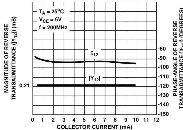
FIGURE 18. REVERSE TRANSADMITTANCE ( $Y_{12}$ ) VS COLLECTOR CURRENT
