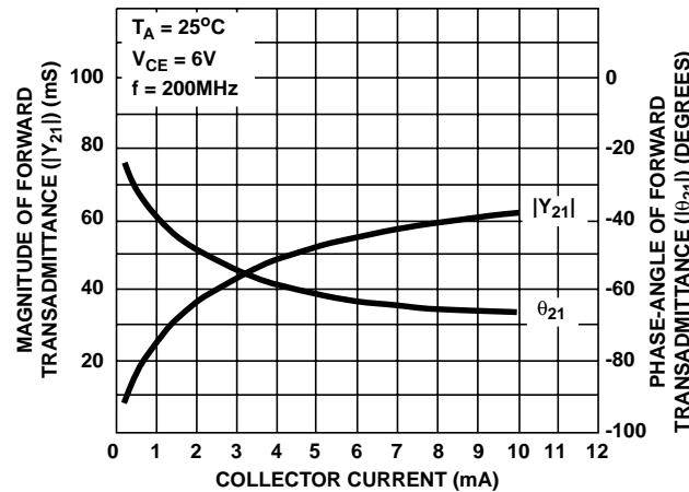
FIGURE 16. FORWARD TRANSADMITTANCE ( $Y_{21}$ ) VS COLLECTOR CURRENT
