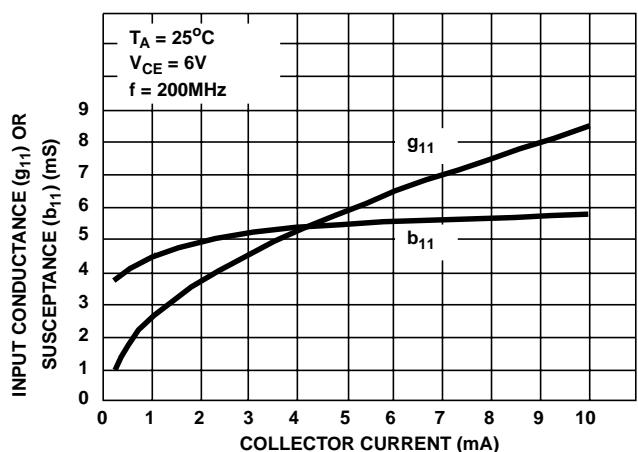
FIGURE 13. INPUT ADMITTANCE ( $Y_{11}$ ) vs COLLECTOR CURRENT
