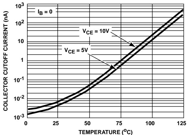
FIGURE 1.  $I_{CEO}$  VS TEMPERATURE FOR ANY TRANSISTOR
