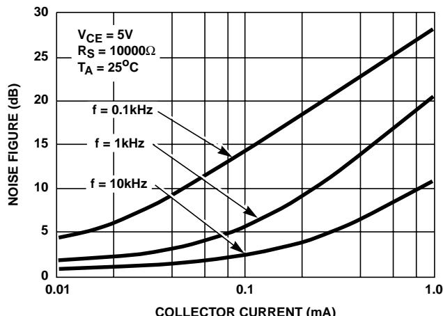
FIGURE 11. NF vs  $I_C$  AT  $R_S = 10\text{k}\Omega$
