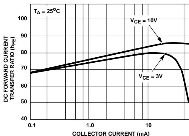
FIGURE 22.  $h_{FE}$  vs  $I_C$  FOR ANY TRANSISTOR
