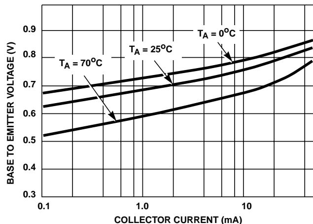
FIGURE 23.  $V_{BE}$  vs  $I_C$  FOR ANY TRANSISTOR
