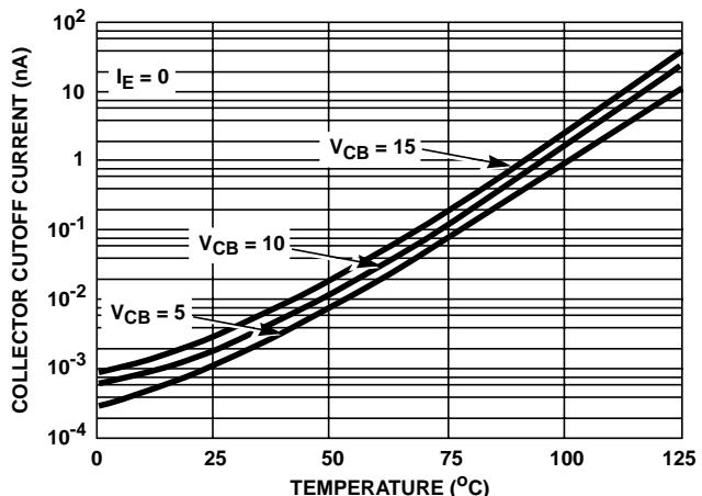
FIGURE 2.  $I_{CBO}$  VS TEMPERATURE FOR ANY TRANSISTOR
