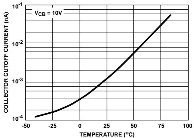
FIGURE 20.  $I_{CBO}$  vs TEMPERATURE FOR ANY TRANSISTOR
