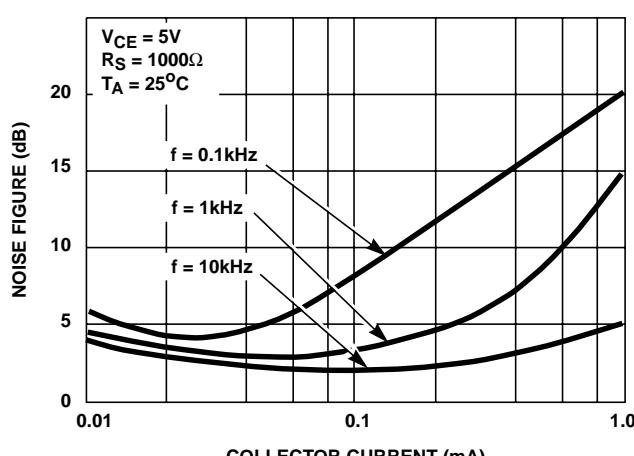
**FIGURE 9. NF vs  $I_C$  AT  $R_S = 500\Omega$**
