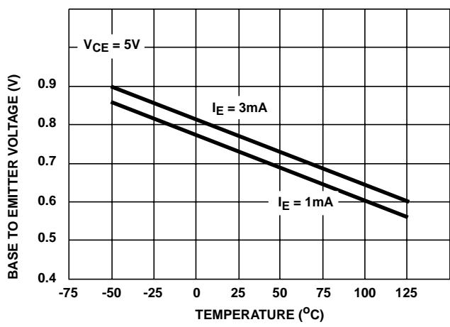
FIGURE 4.  $V_{BE}$  VS TEMPERATURE FOR ANY TRANSISTOR
