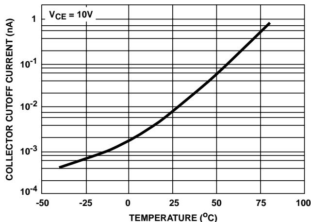
FIGURE 19.  $I_{CEO}$  vs TEMPERATURE FOR ANY TRANSISTOR
