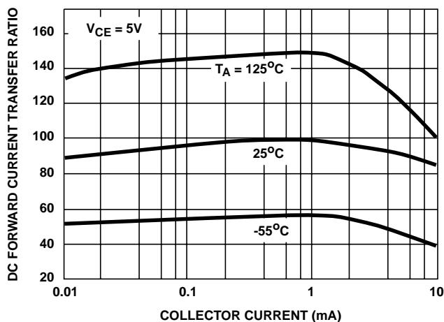
FIGURE 3.  $h_{FE}$  VS  $I_C$  FOR ANY TRANSISTOR
