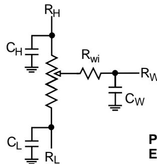
Potentiometer Equivalent Circuit
