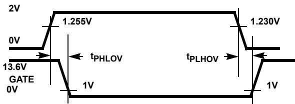
FIGURE 3A. OV TO GATE TIMING
