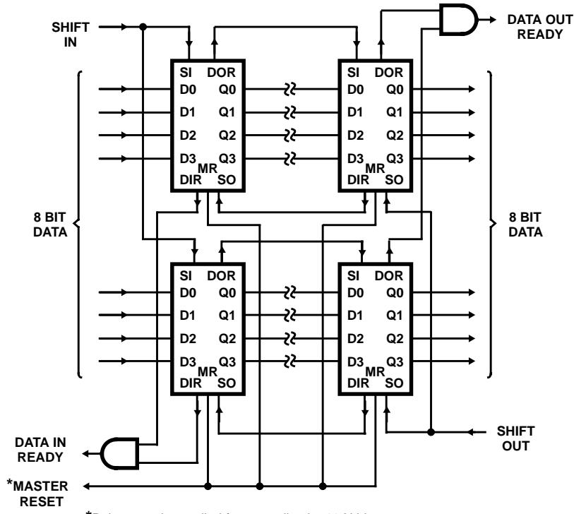
FIGURE 11. EXPANSION, 8-BITS-WIDE-BY-16 N-BITS LONG USING CD40105BMS
