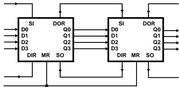
FIGURE 9. EXPANSION, 4-BITS WIDE-BY-16 N-BITS LONG
