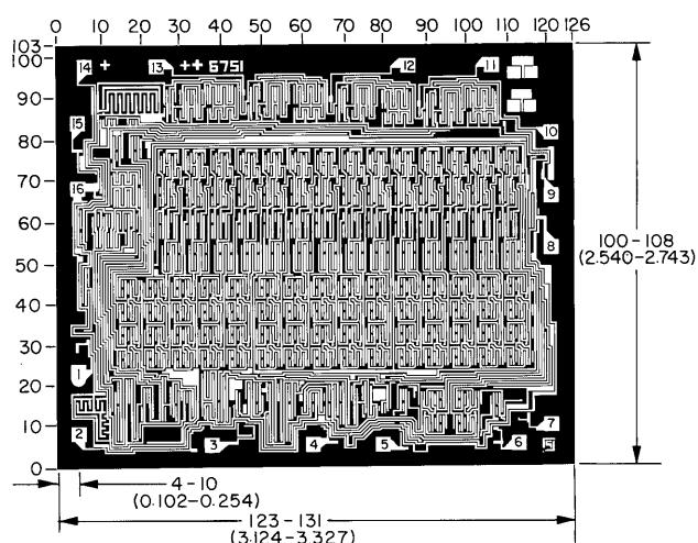
Dimensions in parenthesis are in millimeters and are derived from the basic inch dimensions as indicated. Grid graduations are in mils (10-3 inch).
