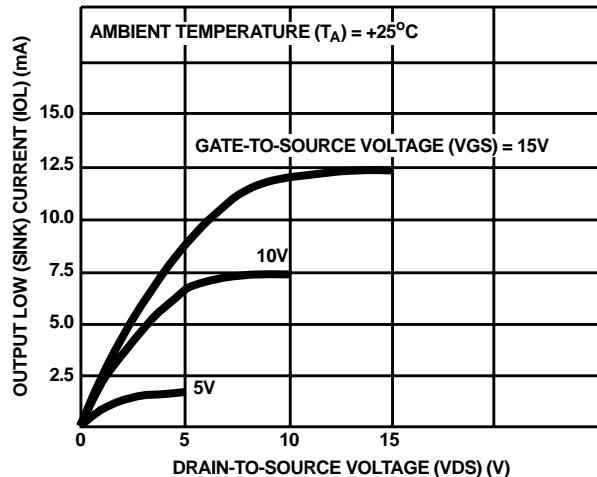
FIGURE 3. MINIMUM OUTPUT LOW (SINK) CURRENT CHARACTERISTICS
