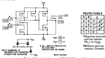
Fig.1 - Schematic diagram of CD40107B (one of 2 gates)
