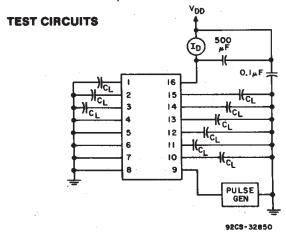
Fig. 11 - Dynamic power dissipation test circuit.
