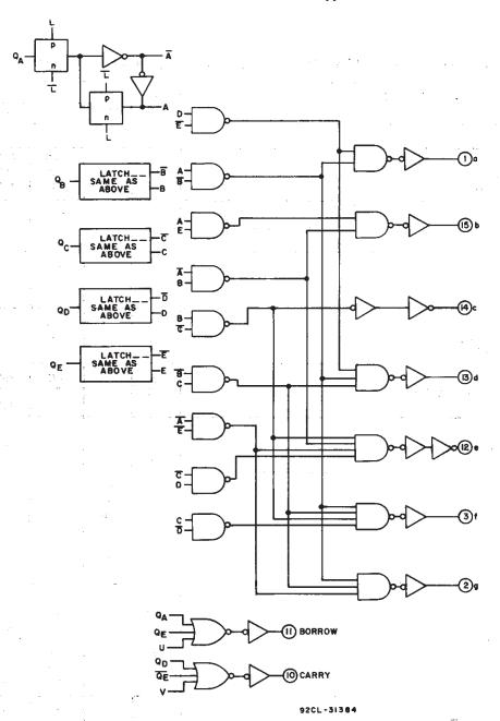
Fig. 2 - Logic diagram with flip-flop and output-driver details.
