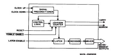
Fig. 1 - Functional diagram.
