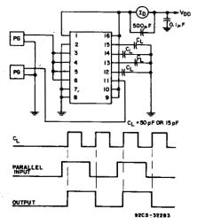
Fig. 10—Dynamic power dissipation test circuit.
