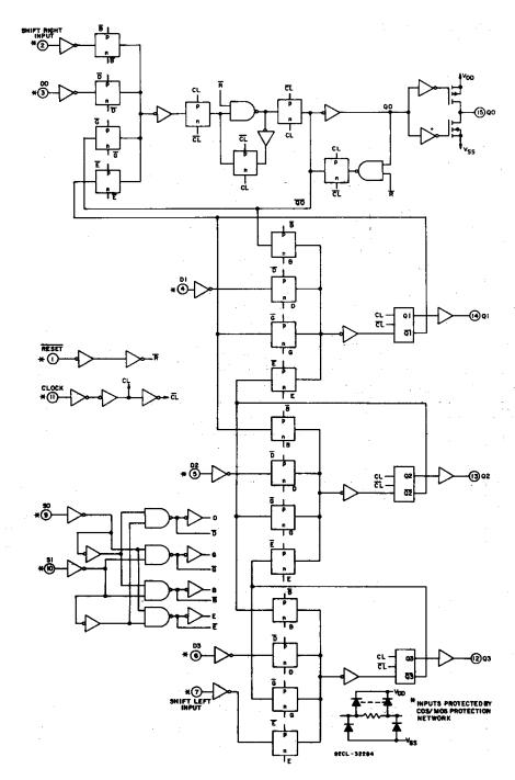
Fig. 8-CD40194B logic diagram.
