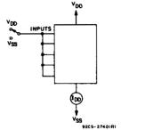
Fig. 11—Quiescent-device-current test circuit.
