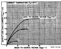
Minimum n-channel output low (sink) current characteristics.
