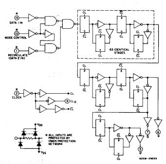
Fig. 1 — Logic diagram.
