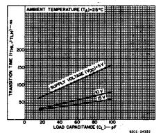
Fig. 8 — Typical transition time as a function of load capacitance (except Q, t<sub>THL</sub>).
