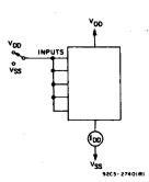
Fig. 13 — Quiescent-devicecurrent test circuit.
