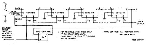
Fig. 14 - Cascading using delayed clocking for reduced clock drive requirements.
