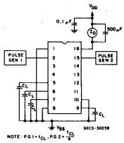
Fig. 11 - Dynamic power dissipation test circuit.
