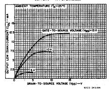
Fig. 3 — Minimum output low (sink)
