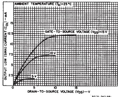
Fig. 3 – Minimum output low (sink) current characteristics.
