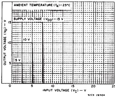
Fig. 9 - Typical voltage transfer characteristics (NAND output).
