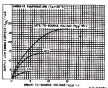
Fig. 2 — Typical output low (sink) current characteristics.
