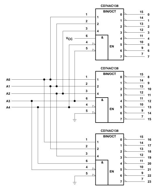
Figure 2. 24-Bit Decoding Scheme
