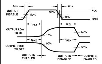
FIGURE 8. HC THREE-STATE PROPAGATION DELAY WAVEFORM
