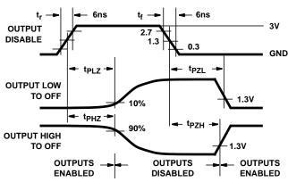
FIGURE 9. HCT THREE-STATE PROPAGATION DELAY WAVEFORM
