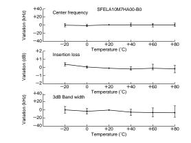
•The SFELA10M7 and SFTLA10M7 series are of input/output symmetric structure so that in theory there is no input/output directionality. Actual circuits may use different input/output loading conditions (for example, mismatched impedance) or capacitance load. In such cases, the waveform will be a little changed by the direction of the input/output of the ceramic filters.
