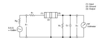
$\begin{array}{l} Rg=50\Omega \quad R_{1}=280\Omega\pm 5\% \quad R_{2}=330\Omega\pm 5\% \\ C_{2}=10\pm 2\ pf \ (Including stray capacitance and Input capacitance \\ of RF Vot Meter) \\ E_{1}:S.S.G. \quad S.S.G. \ Output Voltage \end{array}$
