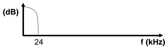
Figure 26. Spectrum After Continuous Time Filter
