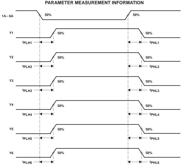
NOTE A: Output skew,  $t_{Sk(0)}$ , is calculated as the greater of: - The difference between the fastest and slowest of  $t_{PLLn}$  (n = 1, 2, ..., 6) - The difference between the fastest and slowest of  $t_{PLHn}$  (n = 1, 2, ..., 6)
