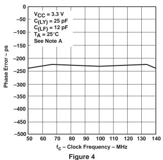
NOTE A: Trace feedback length FBOUT to FBIN = 5 mm,  $Z_O$  = 50  $\Omega$
