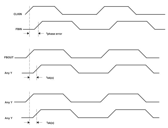
Figure 2. Phase Error and Skew Calculations
