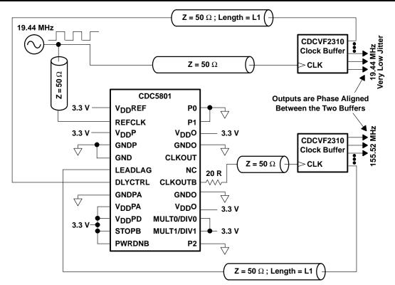
Figure 9. Using the CDC5801 Device as a Multiplier by 8 and Aligning Two Different Clocks
