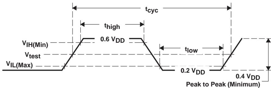
NOTE: All parameters in Figure 4 are according to PCI-X 1.0 specifications.
