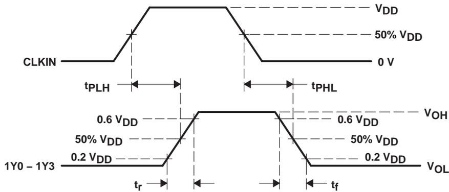
**Figure 2. Voltage Thresholds for Propagation Delay ( $t_{pd}$ ) Measurements**
