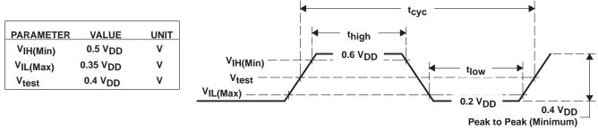
NOTE: All parameters in Figure 4 are according to PCI-X 1.0 specifications.
