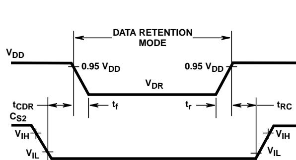
FIGURE 3. LOW  $V_{DD}$  DATA RETENTION TIME WAVEFORMS
