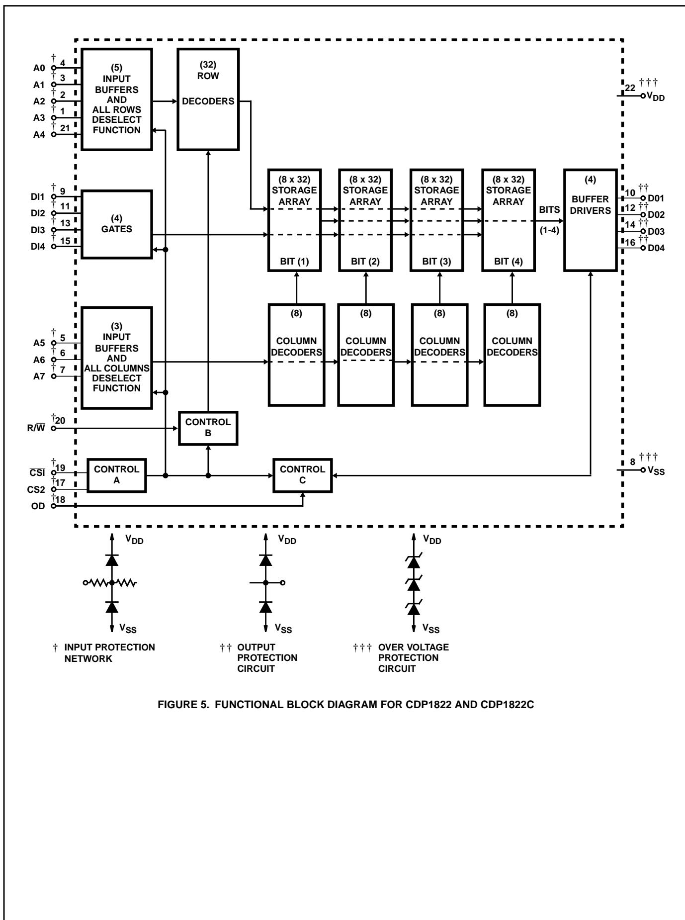
FIGURE 5. FUNCTIONAL BLOCK DIAGRAM FOR CDP1822 AND CDP1822C
