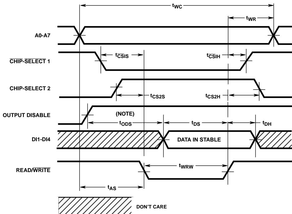
NOTE:  $t_{ODS}$  is required for common I/O operation only. For separate I/O operations, output disable is don't care.
