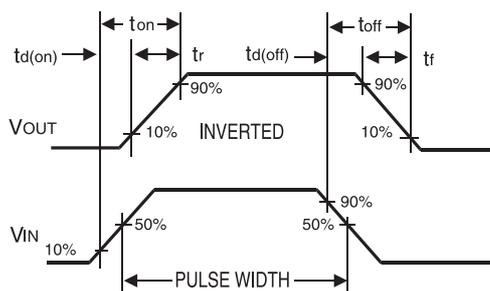
Figure 12. Switching Waveforms
