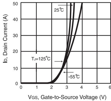
Figure 2. Transfer Characteristics
