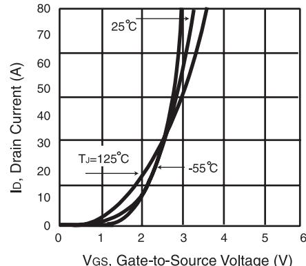
Figure 2. Transfer Characteristics
