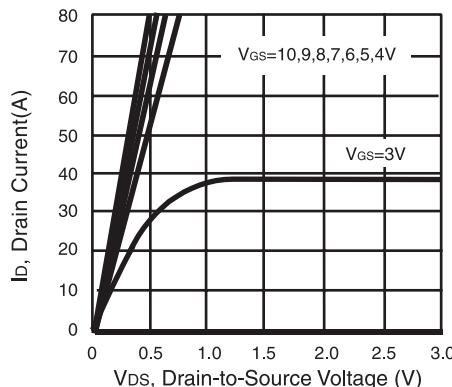
Figure 1. Output Characteristics
