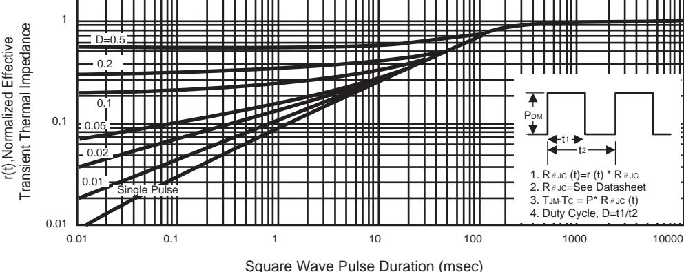
**Figure 13. Normalized Thermal Transient Impedance Curve**
