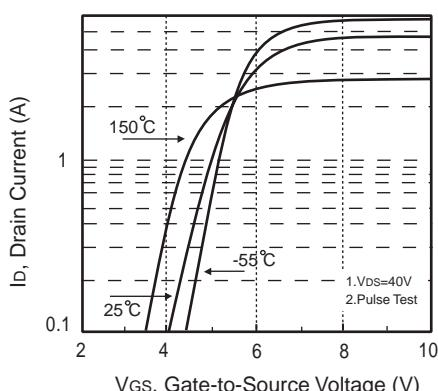
Figure 2. Transfer Characteristics
