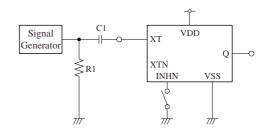
2Vp-p, 10MHz sine wave input signal
