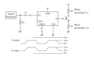
2Vp-p, 10MHz sine wave input signal
