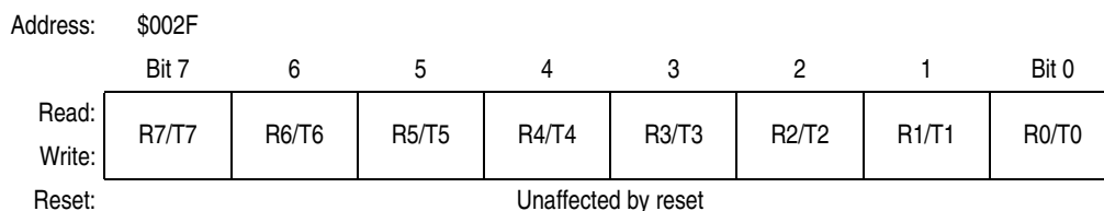
Figure 6-3. SCI Data Register (SCDR)
