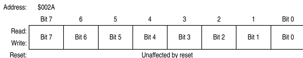
Figure 7-5. SPI Data I/O Register (SPDR)
