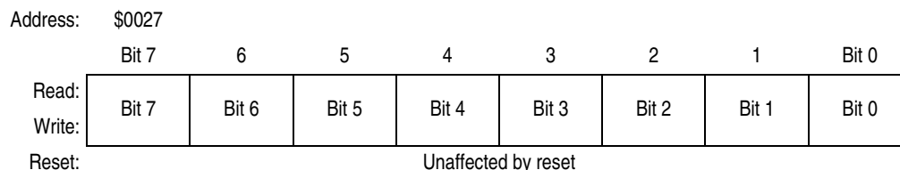
Figure 8-21. Pulse Accumulator Count Register (PACNT)
