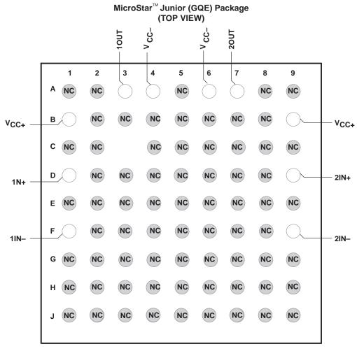
NOTE: Shaded terminals are used for thermal connection to the ground plane.
