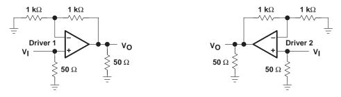
Figure 1. Input-to-Output Crosstalk Test Circuit
