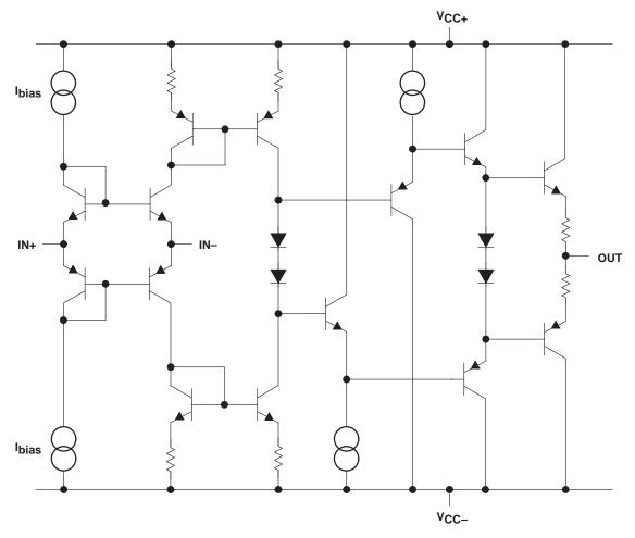
The THS6022 contains two independent operational amplifiers. These amplifiers are current feedback topology amplifiers made for high-speed operation. They have been specifically designed to deliver the full power requirements of ADSL and therefore can deliver output currents of at least 200 mA at full output voltage.
