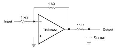
Figure 55. Driving a Capacitive Load
