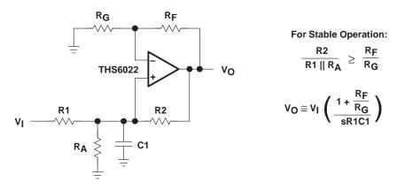
Figure 64. Noninverting CFB Integrator
