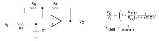
Figure 61. Single-Pole Low-Pass Filter
