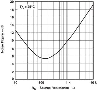
Figure 52. Noise Figure vs Source Resistance
