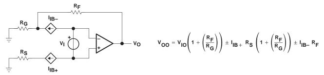
Figure 50. Output Offset Voltage Model
