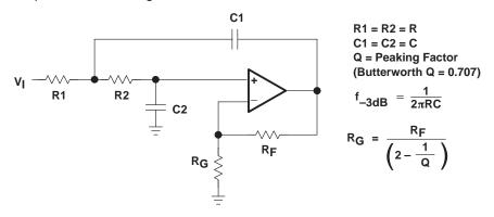
Figure 62. 2-Pole Low-Pass Sallen-Key Filter
