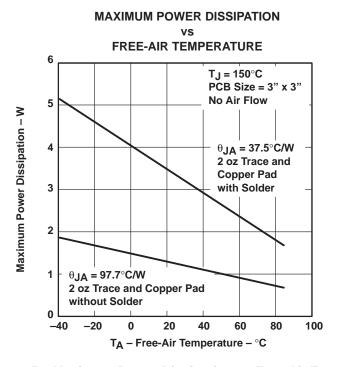
Figure 59. Maximum Power Dissipation vs Free-Air Temperature
