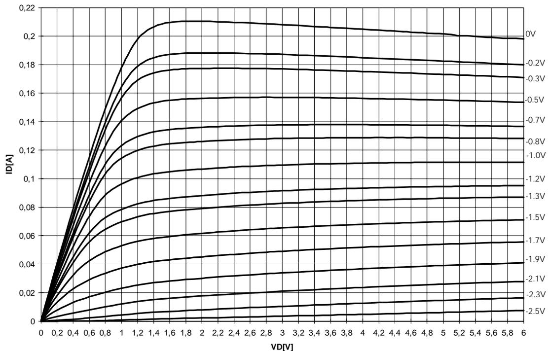
Input characteristics - typical measured values of stage 3, VD3 = 3V
