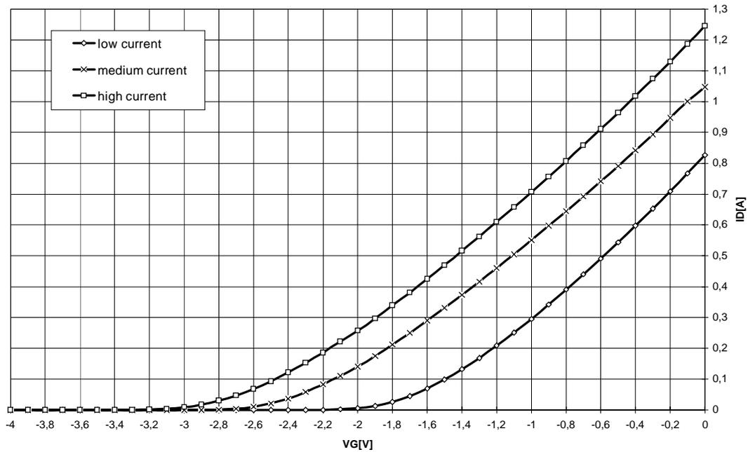
Output characteristics - typical measured values of stage 3
