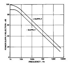
Figure 19. Power Supply Rejection vs. Frequency (AD848)
