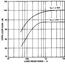
Figure 8. Open Loop Gain vs. Load Resistance (AD849)
