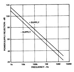
Figure 20. Power Supply Rejection vs. Frequency (AD849)
