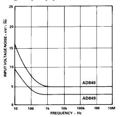
Figure 24. Input Voltage Noise Spectral Density
