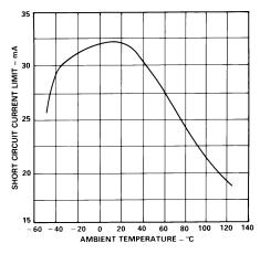
Figure 11. Short Circuit Current Limit vs. Temperature (AD848 and AD849)
