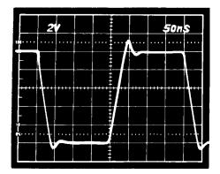
Figure 1a. AD848 Large Signal Pulse Response
