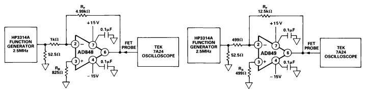
Figure 1. AD848 Inverting Amplifier Configuration
