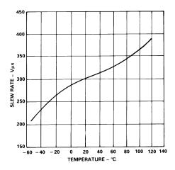
Figure 18. Slew Rate vs. Temperature (AD848 and AD849)
