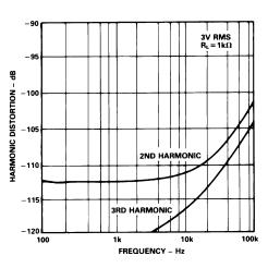
Figure 16. Harmonic Distortion vs. Frequency (AD848)
