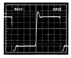
Figure 1b. AD848 Small Signal Pulse Response
