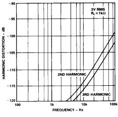
Figure 17. Harmonic Distortion vs. Frequency (AD849)
