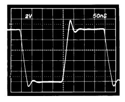
Figure 2a. AD849 Large Signal Pulse Response
