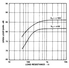
Figure 7. Open Loop Gain vs. Load Resistance (AD848)
