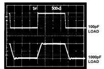
Figure 23 AD848 Driving a Canacitive Load
