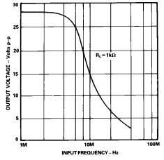
Figure 5. Large Signal Frequency Response (AD848 and AD849)
