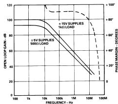
Figure 14. Open Loop Gain and Phase Margin vs. Frequency (AD849)
