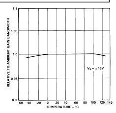
Figure 15. Normalized Gain Bandwidth Product vs. Temperature (AD848 and AD849)
