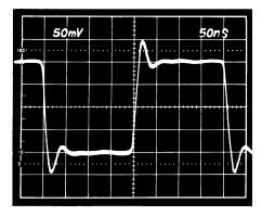
Figure 2b. AD849 Small Signal Pulse Response
