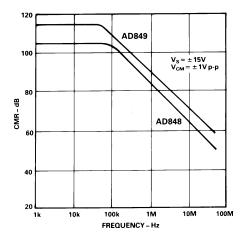
Figure 21. Common-Mode Rejection vs. Frequency
