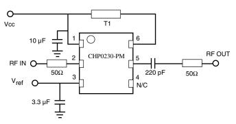
T1 line is important to ensure best bypassing. Optimum performance is achieved through an electrical length of 20°min. at 835 MHz.
