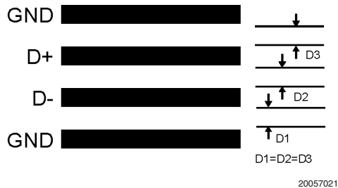
FIGURE 10. Ideal Diode Trace Layout
