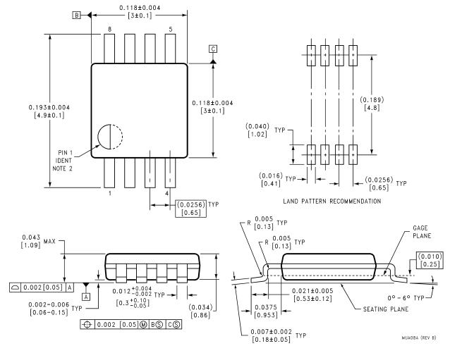
8-Lead (0.150" Wide) Molded Mini Small Outline Package (MSOP), JEDEC Registration Number MO-187 (variation AA), Order Number LM77CIMM-3, LM77CIMMX-3, LM77CIMM-5 or LM77CIMMX-5 NS Package Number MUA08A
