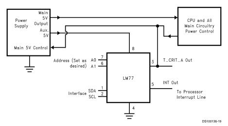
FIGURE 10. ACPI Compatible Terminal Alarm Shutdown. By powering the LM77 from auxiliary output of the power supply, a non-functioning overheated computer can be powered down to preserve as much of the system as possible.
