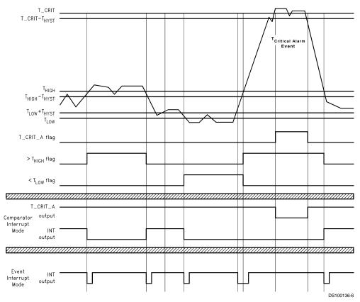
Note: Event Interrupt mode is drawn as if the user is reading the part. If the user doesn't read, the outputs would go low and stay that way until the LM77 is read.
