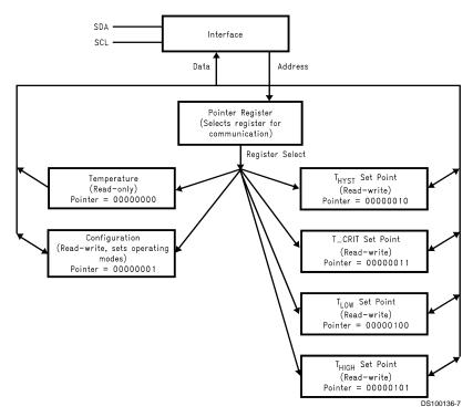
There are four data registers in the LM77, selected by the Pointer register. At power-up the Pointer is set to "00"; the location for the Temperature Register. The Pointer register latches the last location it was set to. In Interrupt Mode, a read from the LM77 resets the INT output. Placing the device in Shutdown mode resets the INT and T\_CRIT\_A outputs. All registers are read and write, except the Temperature register which is read only.
