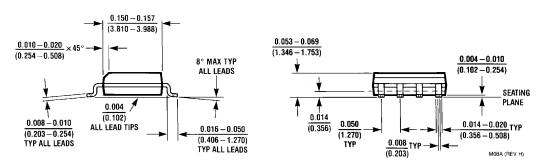
8-Lead (0.150" Wide) Molded Small Outline Package (SOP), JEDEC Registration Number MS-012 (variation AA), Order Number LM77CIM-3, LM77CIMX-3, LM77CIM-5 or LM77CIMX-5 NS Package Number M08A
