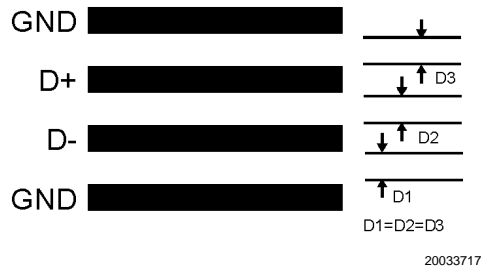
FIGURE 15. Ideal Diode Trace Layout
