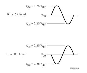
FIGURE 2. The ADC10D040 is designed for use with differential signals of 1.4  $V_{P-P}$  with a common mode voltage of 1.5V. The signal swing should not cause any pin to experience a swing more than 300 mV beyond the supply rails.
