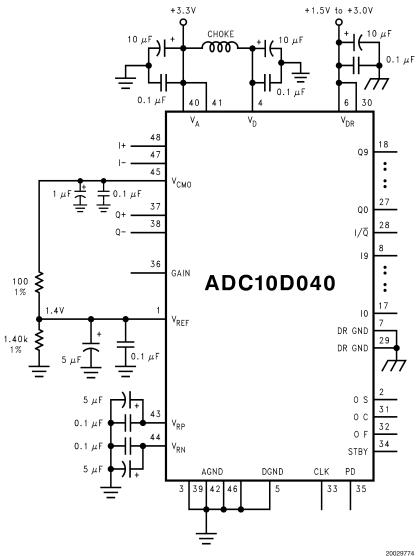
FIGURE 7. The V<sub>CMO</sub> output pin may be used as an internal reference source if its output is not loaded excessively.
