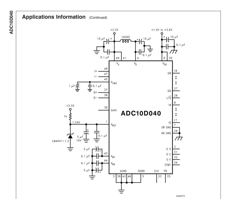
FIGURE 5. Improved Low Component Count Reference Biasing
