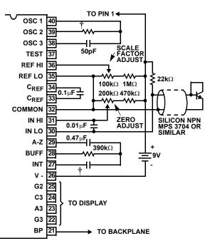
A silicon diode-connected transistor has a temperature coefficient of about  $-2mV/^{O}C$ . Calibration is achieved by placing the sensing transistor in ice water and adjusting the zeroing potentiometer for a 000.0 reading. The sensor should then be placed in boiling water and the scale-factor potentiometer adjusted for a 100.0 reading. † Value depends on clock frequency.
