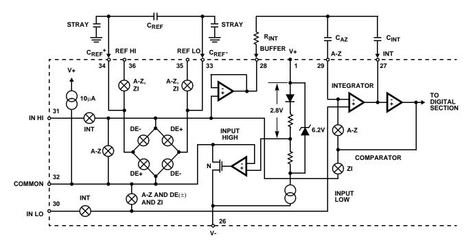
FIGURE 2. ANALOG SECTION OF ICL7136
