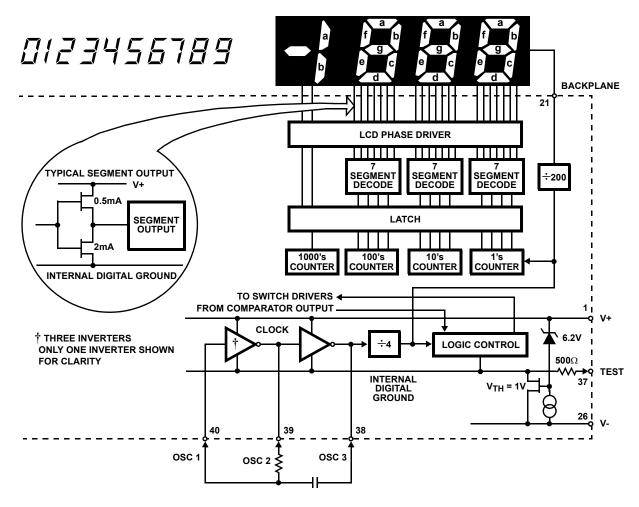
FIGURE 6. ICL7136 DIGITAL SECTION
