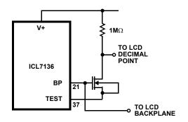
FIGURE 4. SIMPLE INVERTER FOR FIXED DECIMAL POINT
