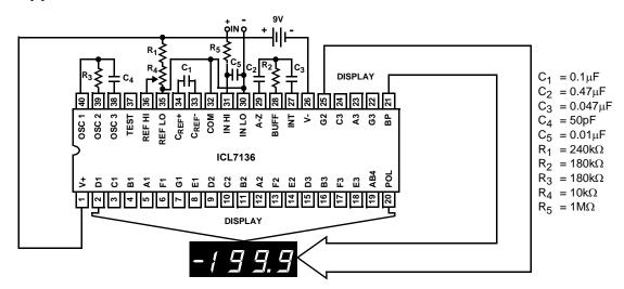
FIGURE 1. ICL7136 TEST CIRCUIT AND TYPICAL APPLICATION WITH LCD DISPLAY COMPONENTS SELECTED FOR 200mV FULL SCALE
