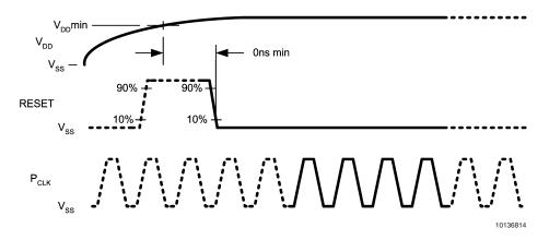
FIGURE 5. Power-On Reset Sequence with Manual Reset
