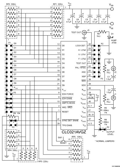
Connect LOCK DETECT to TPG ENABLE for test pattern generator function. Remove RP1 & RP3 and replace RP2 & RP4 with  $50\Omega$  resistor packs for coax interfacing. Install RP1-4 when using ribbon cable for input interfacing. This board is designed for use with TTL power supplies only.
