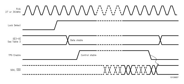
FIGURE 7. Test Pattern Generator Control Sequence
