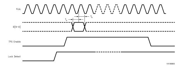
FIGURE 3. Setup and Hold Timing
