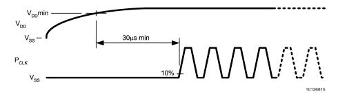
FIGURE 4. Power-On Reset Sequence
