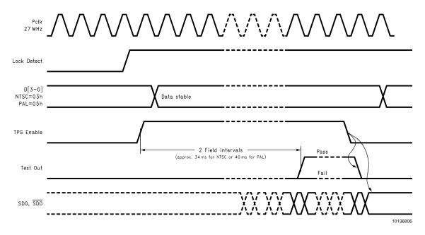
FIGURE 6. Built-In Self-Test Control Sequence
