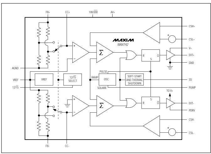
Figure 1. MAX742 Detailed Block Diagram
