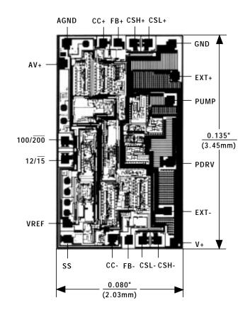
TRANSISTOR COUNT: 375 SUBSTRATE CONNECTED TO V+
