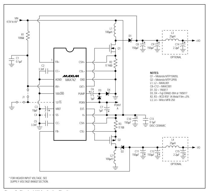
Figure 2. Standard 6W Application Circuit
