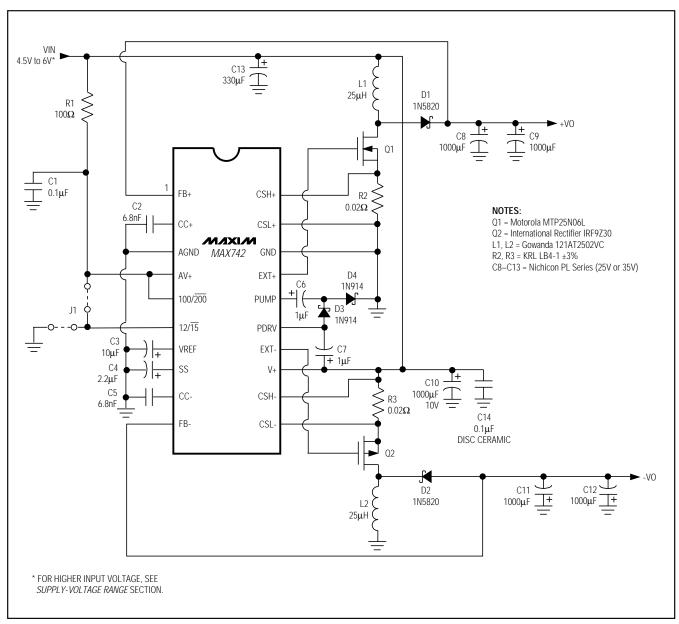
Figure 3. High-Power 22W Application Circuit
