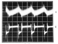
2μs/div A = NOISE WITH i FILTER, 1mV/div B = NOISE WITHOUT FILTER, 20mV/div MEASURED AT -VOUT V + = 5V
