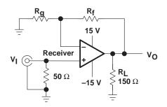
Figure 4. Receiver Test Circuit, Gain =  $1 + (R_f/R_q)$
