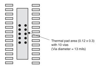
Figure 86. PowerPAD<sup>™</sup> PCB Etch and Via Pattern
