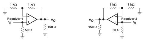
Figure 2. Receiver Input-to-Output Crosstalk Test Circuit
