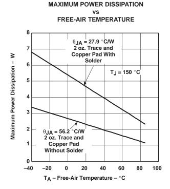
Figure 87. Maximum Power Dissipation vs Free-Air Temperature
