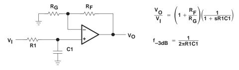
Figure 88. Single-Pole Low-Pass Filter
