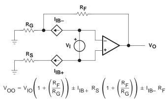
Figure 81. Output Offset Voltage Model
