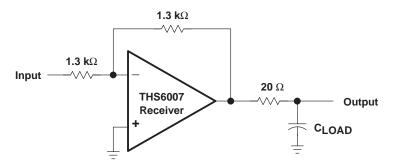
Figure 91. Driving a Capacitive Load
