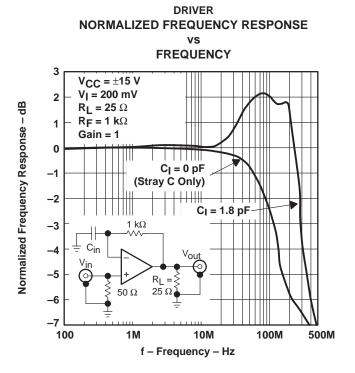
Figure 85. Driver Normalized Frequency Response vs Frequency
