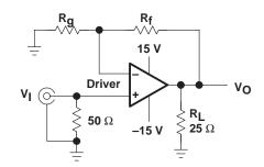
Figure 3. Driver Test Circuit, Gain =  $1 + (R_f/R_q)$
