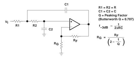
Figure 89. 2-Pole Low-Pass Sallen-Key Filter
