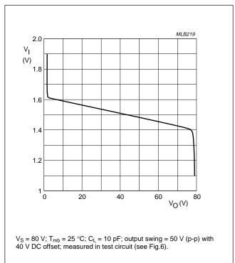
Fig.2 Input voltage at input test-circuit as a function of output voltage; typical values.
