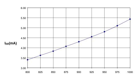
MICRF003 I<sub>DD</sub> vs Frequency (Temperature=25°C, V<sub>DD</sub>=5.0V, SWP Mode)
