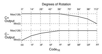
Figure 4. Minor Gauge Outputs
