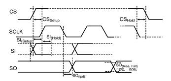
Figure 7. Serial Data Timing Diagram
