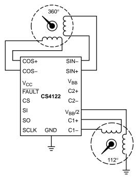
Figure 9. Application with One Minor Gauge
