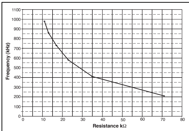
Figure 3: SYNC OUT Frequency vs. FADJ Resistors
