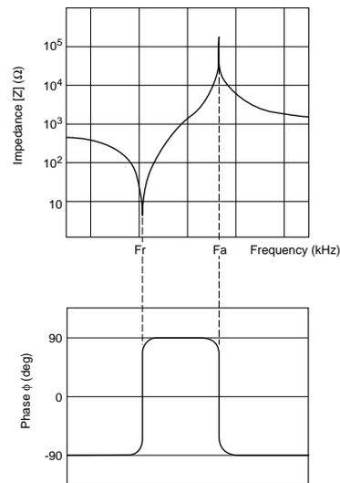
Fig. 2-2 Impedance and Phase Characteristics of CERALOCK®
