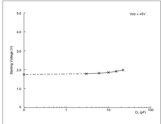
Fig. 5-6 Starting Voltage Characteristics against CL (CL1=CL2)
