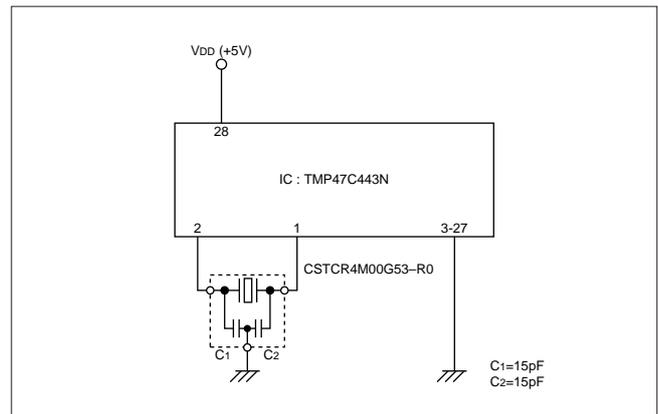
Fig. 6-2 Application to TMP47C443N (TOSHIBA)
