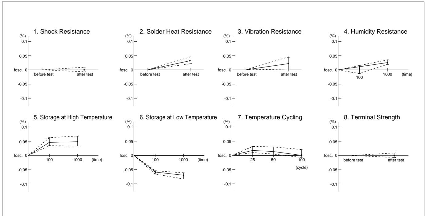
Fig. 3-2 General Changes of Oscillation Frequency in Each Reliability Test (CSTLS4M00G53-B0)
