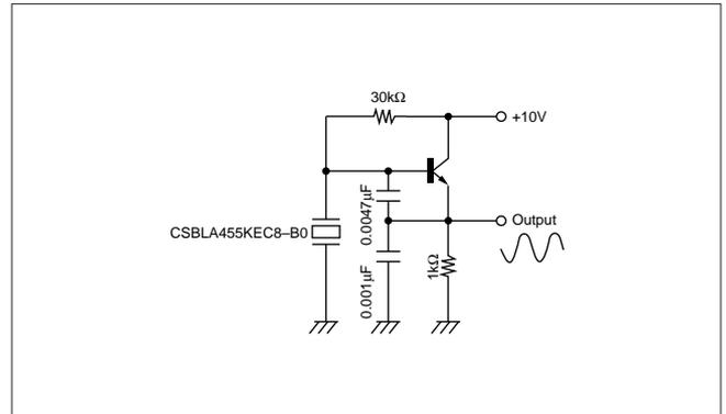
Fig. 4-4 Example of Oscillation Circuit with a Transistor
