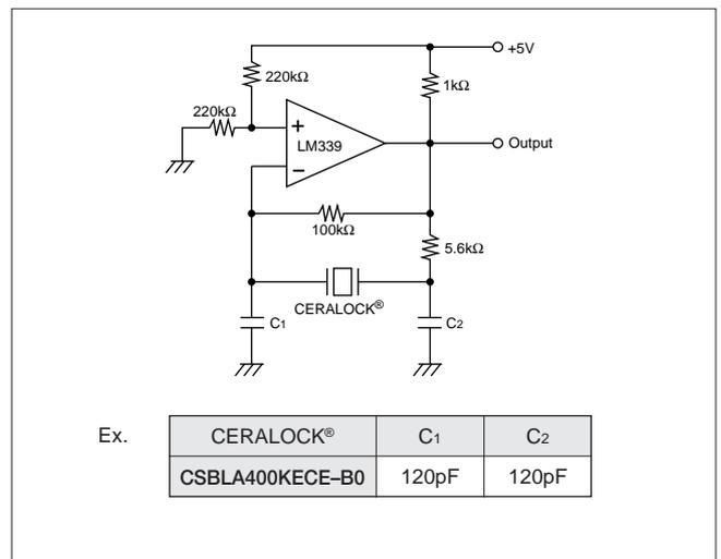
Fig. 4-5 Example of Application to a Comparator
