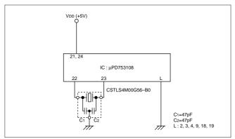
Fig. 6-5 Application to  $\mu$ PD753108 (NEC)
