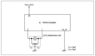
Fig. 6-7 Application to TMP87C809BN (TOSHIBA)
