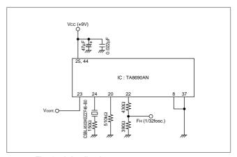
Fig. 6-18 Application to TA8690AN (TOSHIBA)
