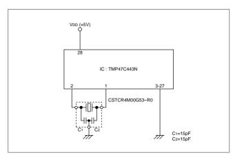
Fig. 6-2 Application to TMP47C443N (TOSHIBA)
