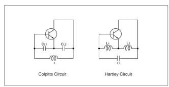
Fig. 2-6 Basic Configuration of LC Oscillation Circuit
