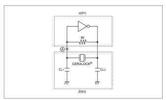
Fig. 2-8 Basic Oscillation Circuit with inverters
