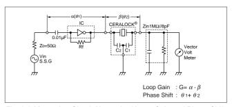
Fig. 2-9 Measuring Circuit Network of Loop Gain and Phase Shift
