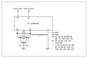
Fig. 6-25 Application to LC895299 (SANYO) (Error Correction of CD-ROM LSI)
