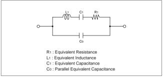
Fig. 2-3 Electrical Equivalent Circuit of CERALOCK®
