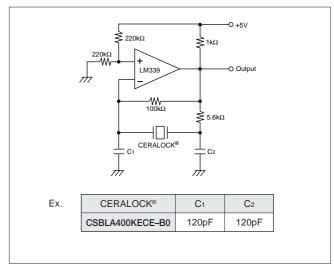
Fig. 4-5 Example of Application to a Comparator
