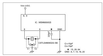
Fig. 6-27 Application to ICs for Voice Synthesis MSM6650GS (OKI)
