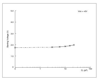
Fig. 5-6 Starting Voltage Characteristics against CL (CL1=CL2) (IC: TC74HCU04, CERALOCK®: CSACW33M8X51-B0)
