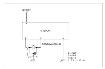
Fig. 6-16 Application to  $\mu$ PD65 (NEC)
