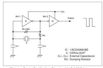
Fig. 4-1 Basic Oscillation Circuit with C-MOS Inverter
