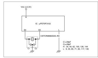
Fig. 6-15 Application to  $\mu$ PD70F3102 (NEC)
