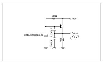
Fig. 4-4 Example of Oscillation Circuit with a Transistor
