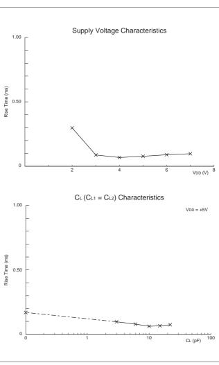
Fig. 5-4 Examples of Characteristics of Oscillation Rise Time (IC: TC74HCU04, CERALOCK®: CSACW33M8X51-B0)
