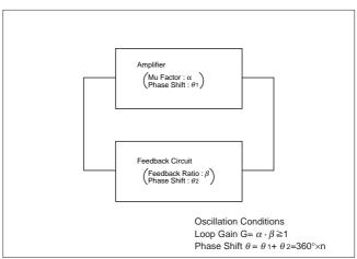
Fig. 2-7 Principle of Oscillation
