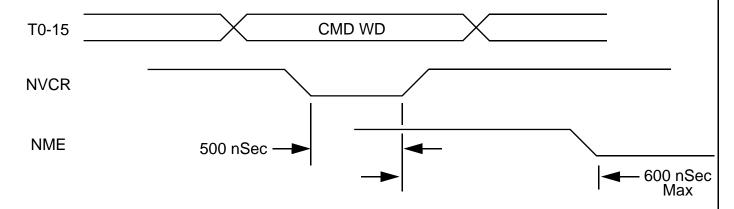
Any message can be illegalized by applying an active low on the NME signal within 600 nSec of the rising edge of NVCR at this time. The RT will respond with a Status word having the Message Error bit set. See Section 1.2.1.1 for implementing the Message Illegalization.
