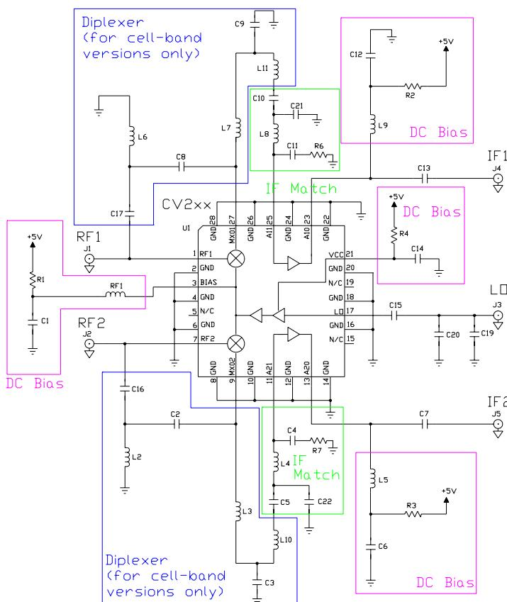
**CV211-3:** The application circuit can be broken up into three main functions as denoted in the colored dotted areas above: RF/IF diphasing (blue), IF amplifier matching (green), and dc biasing (purple). There are various placeholders for chip components in the circuit schematic so that a common PCB can be used for all WJ dual-branch converters. Further details are given in the Application Note located on the website titled "CV2xx Series - PWB Design Guidelines".
