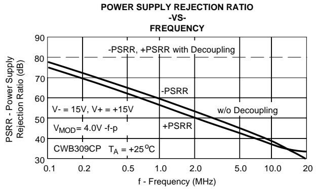
By inserting 1K ohm resistors in series with V+ and V- power supply lines and decoupling both pins at the device socket, it is possible to improve power supply rejection ratios of a video switch by 50dB at frequencies of 20MHz and higher.
