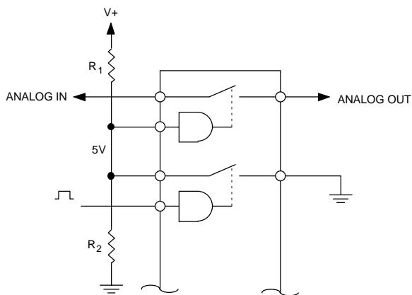
This circuit provides logic inversion with two resistors and one switch. It does not require additional logic parts. The resistors divide the supply voltage down to a 5 volt level when high and are switched to a low level via the switch. This configuration allows a single pole, single throw switch to be changed into a single pole, double throw switch.
